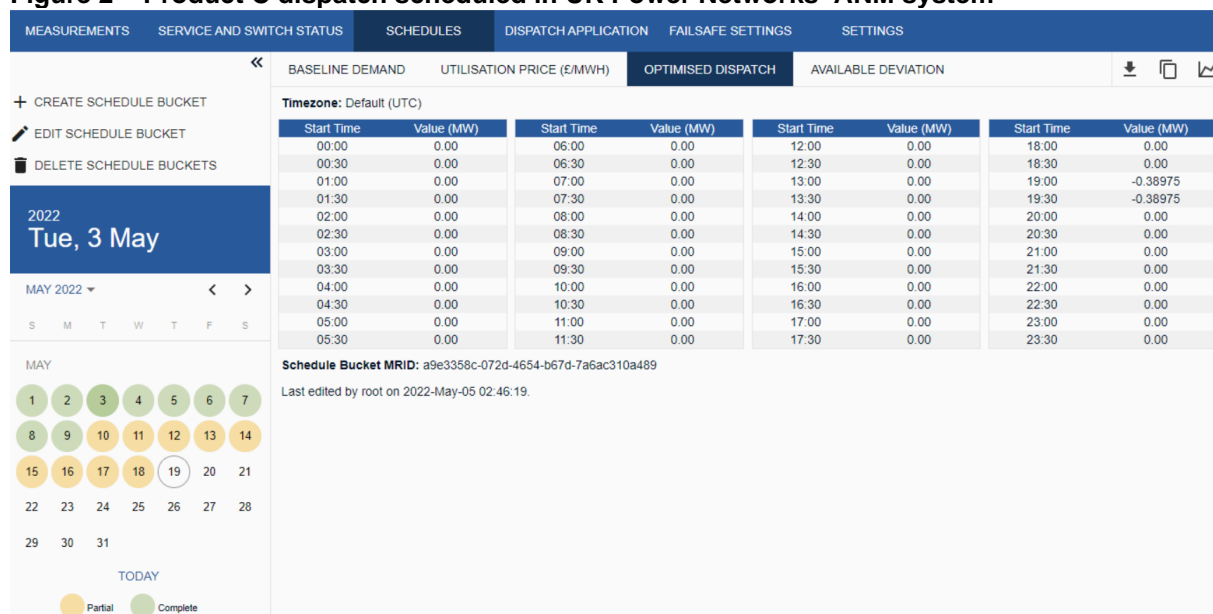
Figure 2 – Product C dispatch scheduled in UK Power Networks' ANM system
