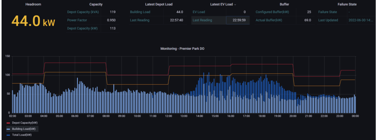
Figure 5 – Dashboard view of depot load
