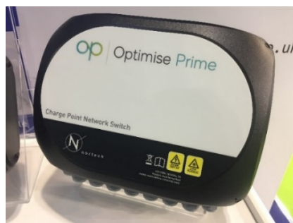
Figure 6 – Charge Point Network Switch, part of the depot solution for WS2
